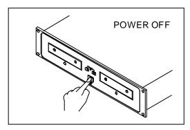
Switch off the power after the disc holder has been closed with the OPEN/CLOSE button.
